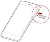
2. Hold the nano-SIM card with the cut corner oriented as shown and slip them into the card holders.
